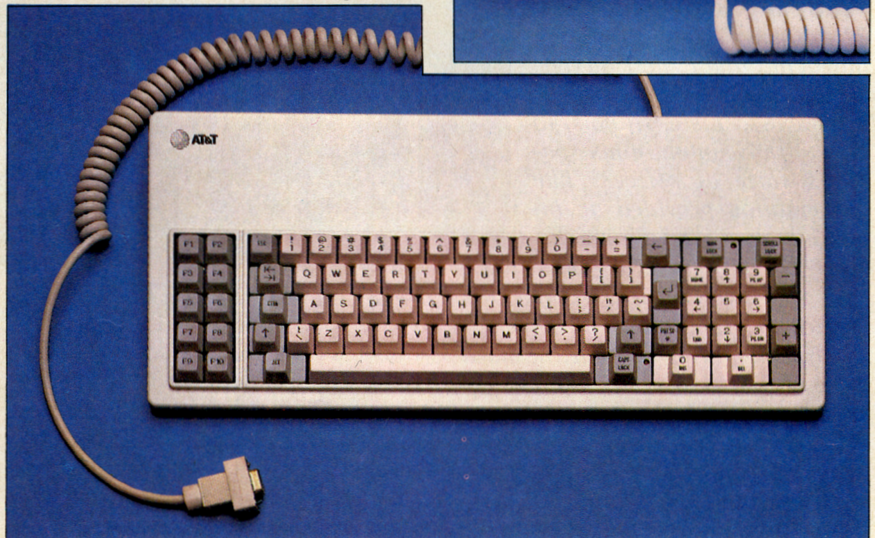
The keyboard has function keys on the left and a numeric/edit keypad on the right. Four-foot cord connects to the back of the keyboard (inset).
