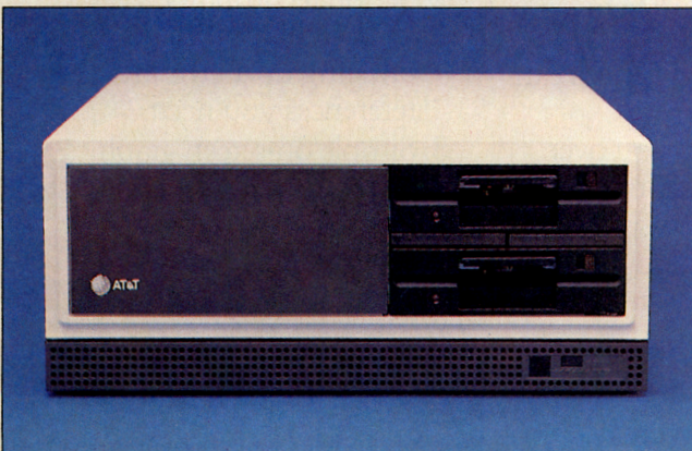
A slimline 5 1/4" floppy disk drive comes with the AT&T Personal Computer. A second floppy drive or hard disk are optional.
