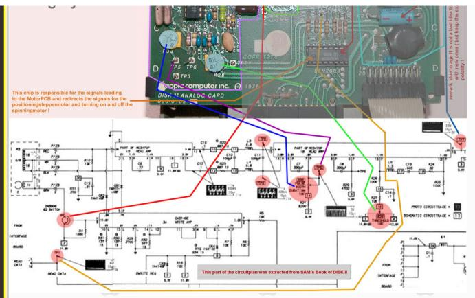
Our attention will be fixed to the 2 variable yellow resistors with the light blue spintops at the bottom of the picture marked as R33 and R 28 ( in the drawing also the one indicated with the blue line and the other marked by the light green line ). Within the circuitplan they are marked by the enlarged red spots.
