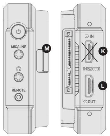
• M. Release Button – press the battery release button on the rear right hand side of the Ninja V/V+ to disengage the AtomXpansion Port.
