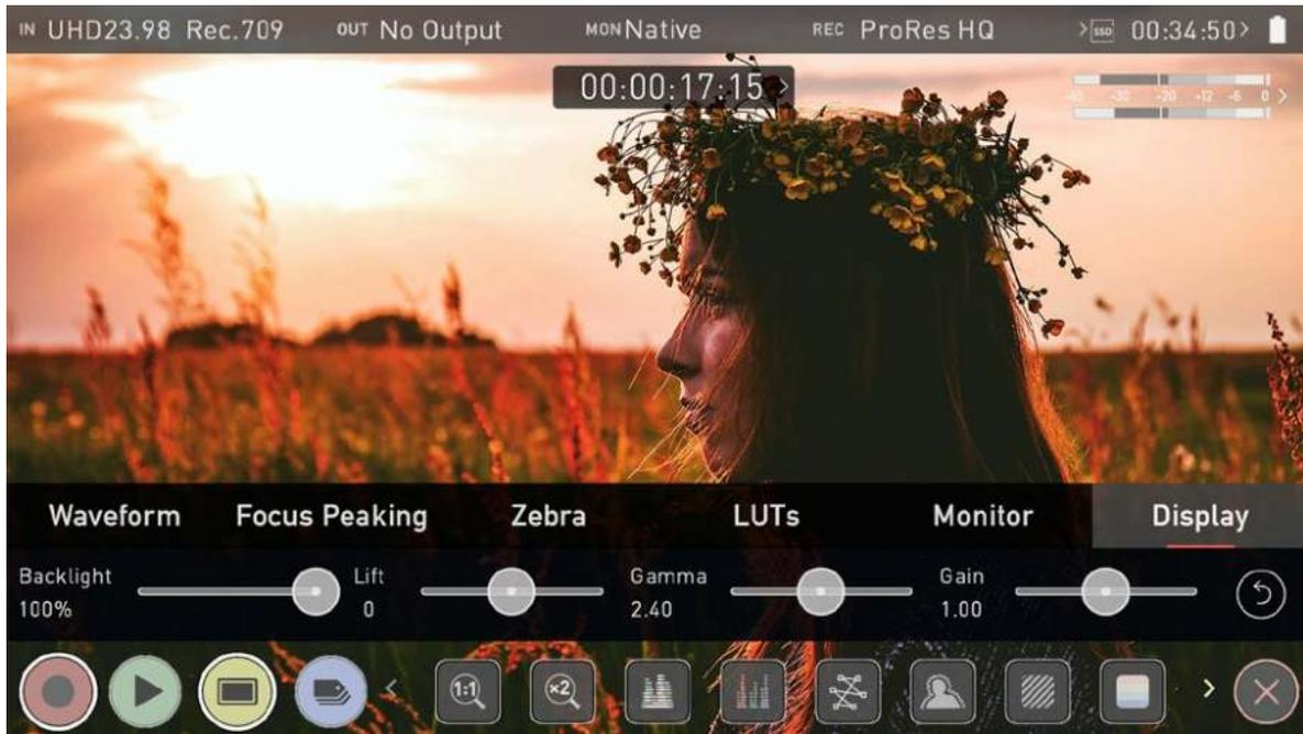
This menu gives you the option to change the screen brightness by adjusting the slider when in Native, Rec709 and LUT mode. As you slide to the right the brightness will increase and when at 100% the image will be using the full 1000nits of the display. As with any electronic screen device increasing the brightness will increase the power draw and battery life will be effected accordingly.
