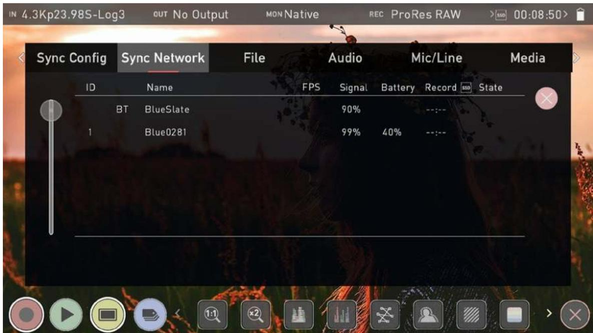
The Sync Network menu page displays all of the devices that you have added to the timecode network. The columns in the table will list the details for each connected device in the sync network.
