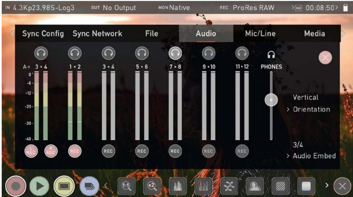
In addition to selecting the Audio tab from the menu tabs across the top of the screen, you can also access the Audio menu by tapping the audio meters (shown below) on the record, monitor and playback home screens.
