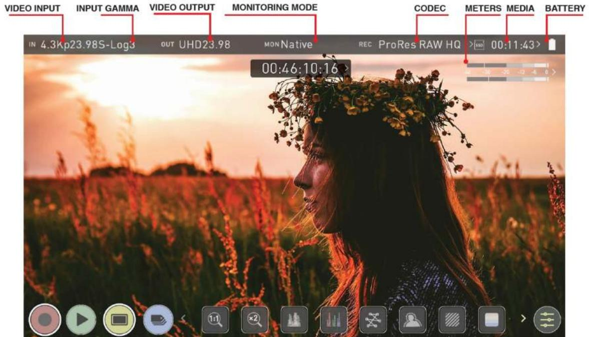
*In the image the NINJA V has an input and an output, and is ready to record the signal or play the last recorded file from disk.*
