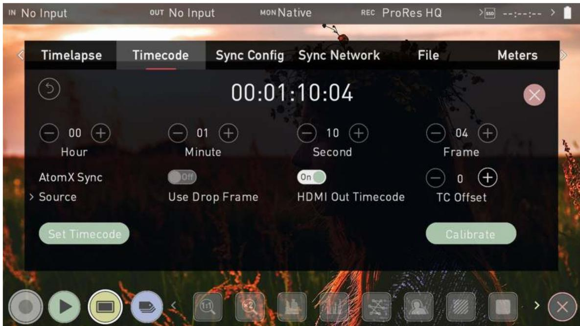
By attaching an optional AtomX SYNC module or Atomos CONNECT to your NINJA V, you can take advantage of ATOMOS AirGlu™ wireless sync technology to simplify your multi-camera productions. These accessories allow for wireless timecode synchronization with other Atomos devices, cameras, audio recorders and timecode systems on set.
