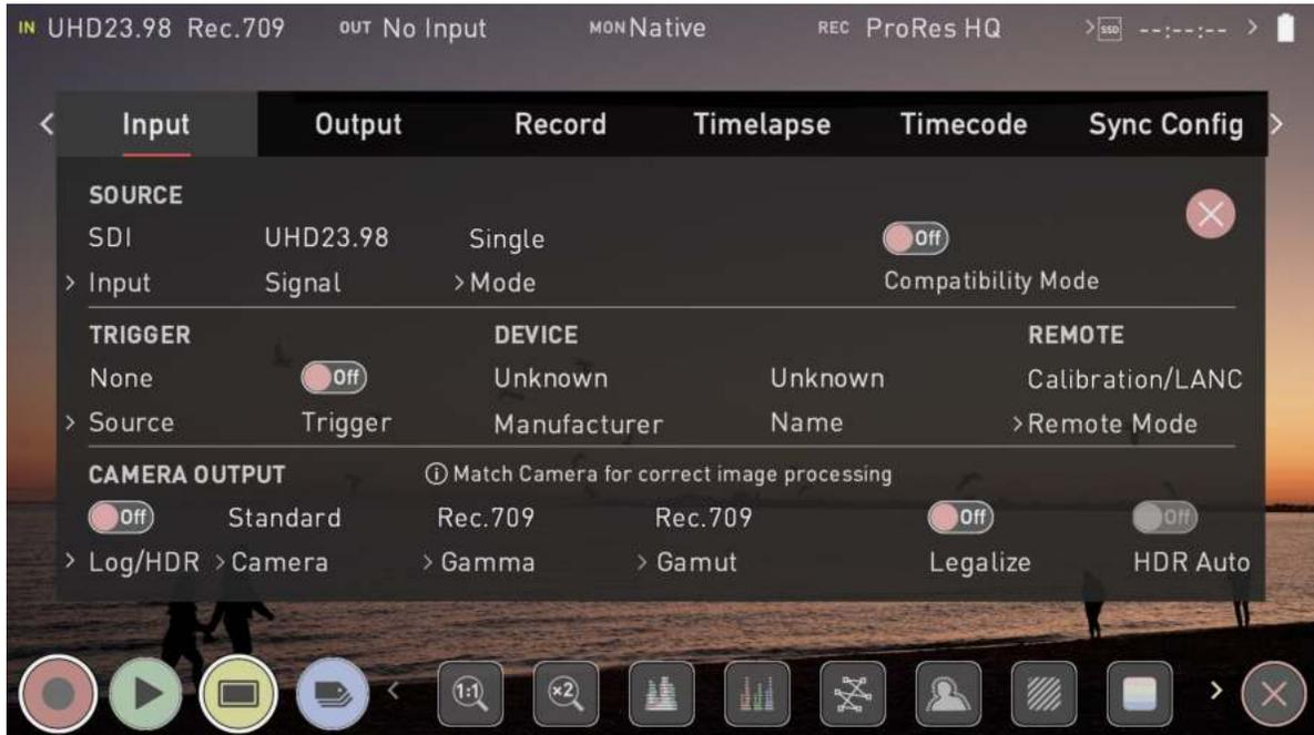
With the ATOMOS CONNECT attached, you will be able to tap on Input in the Input Menu to switch to SDI as your input. The Source Menu will open, where you can select SDI. A note will advise that changing input source will take a few seconds. Tap Ok and wait for your device to switch to SDI source mode. Once in this mode, the input menu will resemble the image shown above.
