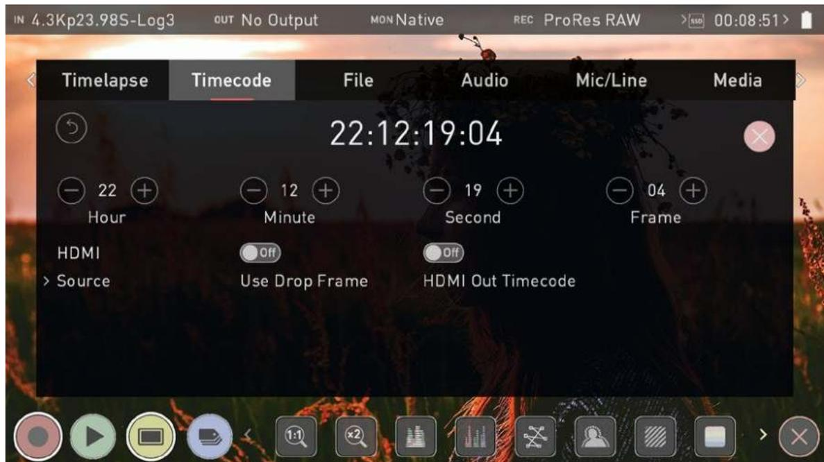
**Timecode Display:** Displays the current timecode. The position of the timecode display will depend on the screen mode you are using. In monitoring mode it appears in the center top, below the info bar. In home screen mode the timecode display sits on the bottom near the REC PLAY MON EDIT icons. Touching the Timecode display will take you to this Timecode menu screen.
