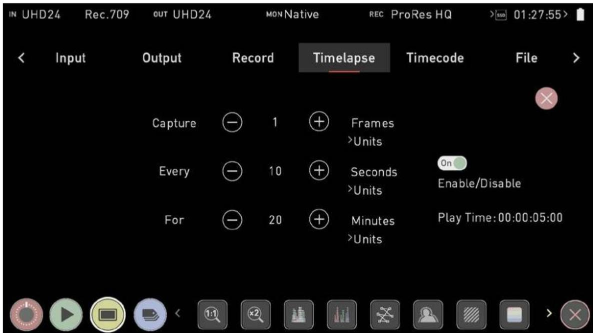
This menu allows you to set up recording of a time-lapse sequence as a single video file in ProRes, DNx or ProRes RAW from an HDMI or SDI source.
