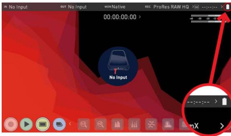
On the Power menu screen press the green Power icon for 4 seconds. **Four seconds** can seem like a long time, but this is intentional to make sure that the NINJA V can't be turned off accidentally.
