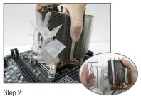
Place the cooler atop the CPU, aligning the four mounting screws with the mounting holes on the ILM. (If your cooler has a fan grill which may cause interference when you tighten the screws, remove it first and replace it after tightening the screws.)
