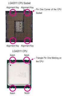
B. Follow the steps below to correctly install the CPU into the motherboard CPU socket.
