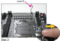
Push the lever closest to the "lock" marking " $\triangle$ " (below referred as lever B) down and away from the socket. Then lift the lever.
