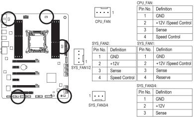
Be sure to connect fan cables to the fan headers to prevent your CPU and system from overheating. Overheating may result in damage to the CPU or the system may hang.
