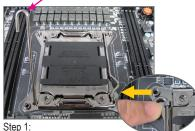
Push the lever closest to the "unlock" marking "
