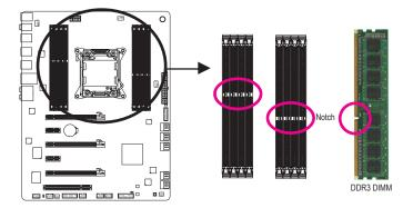
A DDR3 memory module has a notch, so it can only fit in one direction. Follow the steps below to correctly install your memory modules in the memory sockets.
