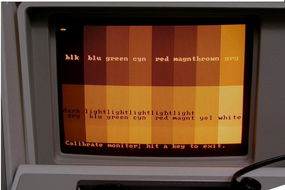
CGACAL PROGRAM AS IT APPEARS ON AMBER MONITOR RUNNING WITH A CGA CARD: NOTE INTERFERENCE ON COLOR BARS FROM CHROMA SUB-CARRIER.
