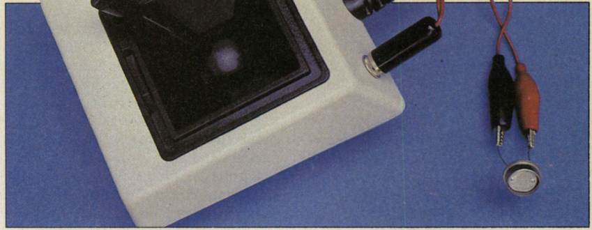
Adding a phone jack to joystick permits using a CdS sensor.
