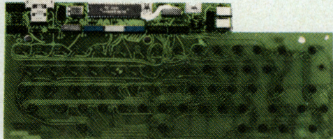
Fig. 17C - A look inside the infrared keyboard. The keys and rubber-domed membrane sheet have been removed to expose the contact points directly in the circuit board (see Fig. 17B)
