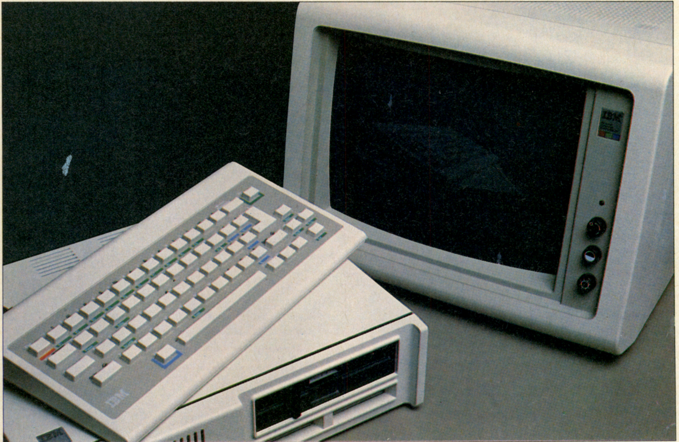
The PCjr is pictured here with the 62-key keyboard on top of the expanded system unit (monitor not included in $1269 price).
