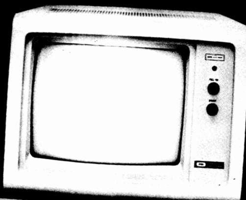
Princeton Graphic Systems HX-12: 12-inch screen, RGB input, dot pitch of .31mm
