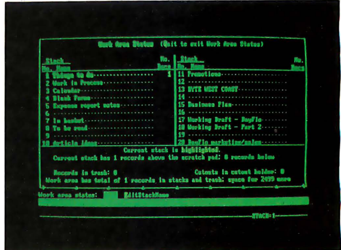
Photo 6: The Work Area Status screen—a map of the Dayflo desktop. Only one record has been entered in the first stack; although some of the other stacks have been named, they're empty until records are either created or pulled from the main database.
