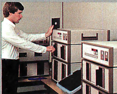
The FORMASTER Series One intelligent diskette duplicator produces up to 326 fully verified copies per hour, with CopyLock™ piracy protection and copy serialization added automatically.
