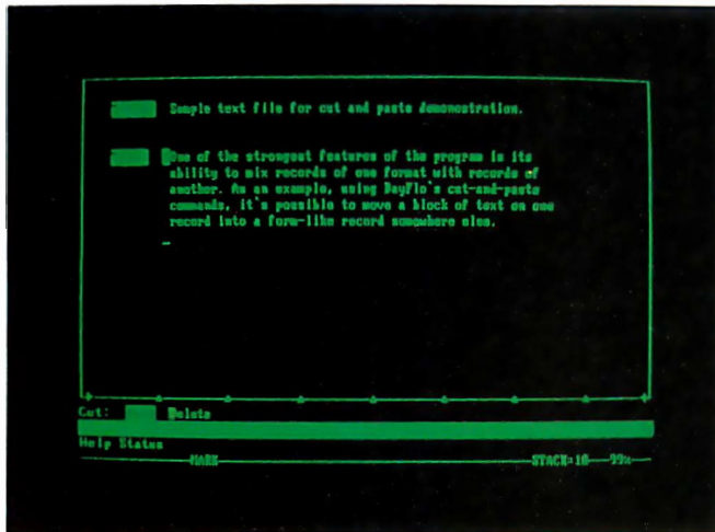
Photo 13: Blocks are stored in the Dayflo "cutout holder" and pasted in where needed. Once a block has been placed in the holder, it remains available for reuse until an active decision is made to throw it away.
