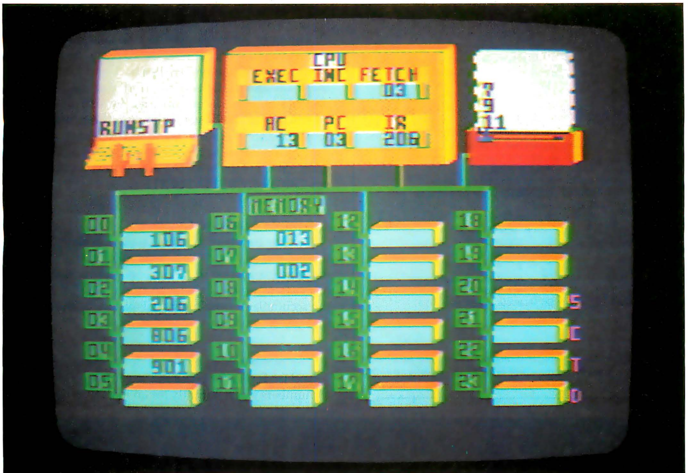
Photo 1: The Simulated Computer's main display, showing (clockwise from upper left) the input device (a terminal), the central processing unit, the output device (a printer), and system memory.
