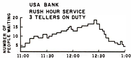
Figure 7: Time plot of the state of a queuing system. The fine resolution of the graphics screen allows compact summaries of the results of a simulation.
