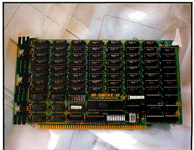
Photo 4: The M-DRIVE/H solid-state disk emulator.
