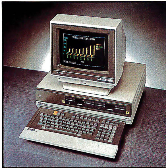
Photo 3: The Sord M68, a 68000-based desktop system. In the spring of 1984, the machine will be available with 1 megabyte of RAM standard, expandable to 4 megabytes, using 256K-bit dynamic RAMs.
