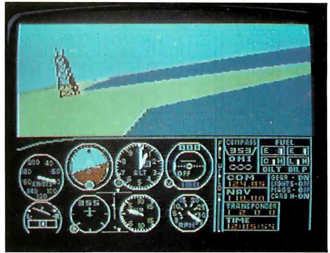
Photo 1: The view forward while waiting for takeoff clearance is shown in 1a. Note the instrument status. Photo 1b shows the situation just after lift-off, banking to the right. Instrument indications correspond to control settings and aircraft speed and attitude.
