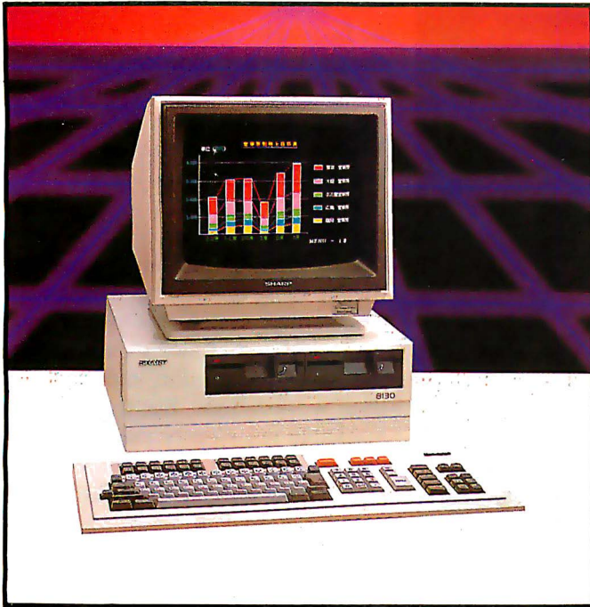
Photo 5: 5a shows Sharp's top-of-the-line office computer, the OA-8100, which employs a 68000 processor and supports Unix System III. 5b shows a TV graphic generated by the Sharp C1 home-graphics processor. Note the palette of shapes at the bottom of the screen. Pictures are created by "picking up" copies of the shapes and positioning them (by cursor movement) at the desired location on the screen. Memos also can be created by picking from a different palette.
