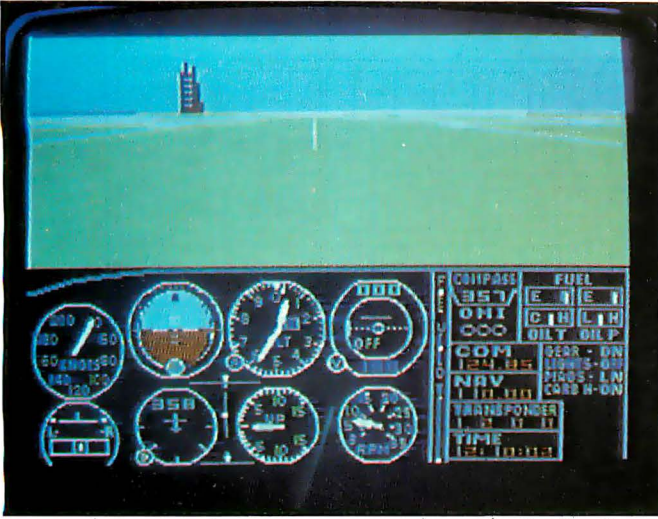
Photo 1: The view forward while waiting for takeoff clearance is shown in 1a. Note the instrument status. Photo 1b shows the situation just after lift-off, banking to the right. Instrument indications correspond to control settings and aircraft speed and attitude.
