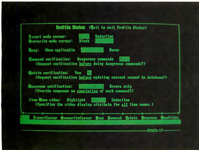
Photo 7: The Profile Status screen shows how the system has been set to respond to errors and dangerous commands. You can change the response settings and some of the major video attributes.
