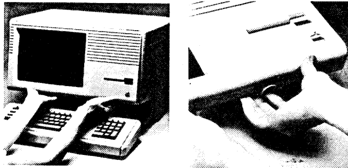
Figure 1 To remove the front panel, feel for the finger grips at the bottom edge and push up gently.
