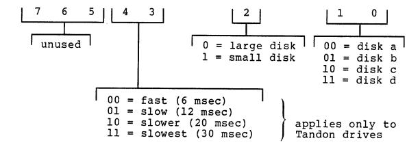
The speeds listed for the table above are the drive stepping rates between tracks.
