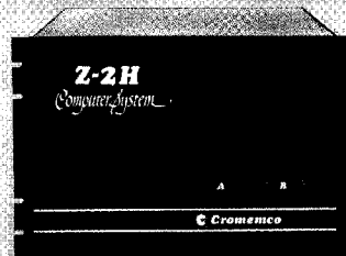
Model Z-2H 11 Megabytes of hard disk storage Up to 512K bytes of RAM/ROM Dual floppy disks
