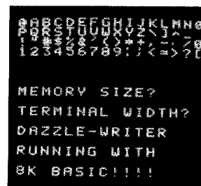
Top four lines show range and style of alphanumeric obtainable with Cromemco's DAZZLE-WRITER software. Query lines are first two prompts from MITS BASIC.
