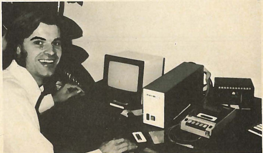
Richard Peterson, president of PolyMorphic Systems, with a complete Poly 88 system (computer, keyboard, TV monitor, cassette recorder).
