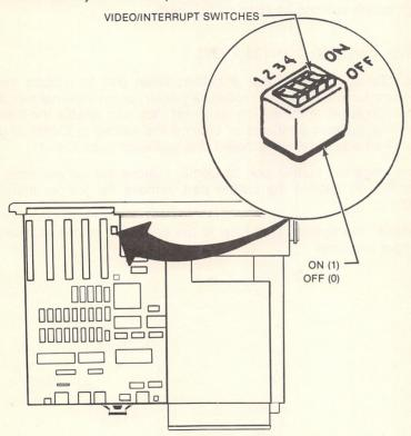
Switch 1 is the Video switch. This switch is set for CGA-type video hardware (either the internal hardware or an optional video board). Set this switch to OFF if you install and use an optional Mono/Text-type video board. If you have a Mono/Text-type board installed, Switch 1 must be ON any time you want to use either the internal CGA video hardware or an optional CGA-type video board. You can change the Video switch setting as often as you wish.
