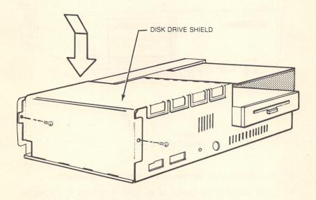
Hold the cover at a slight downward angle to the front of the unit, and guide the cover onto the tracks on the computer chassis. 4. Gently slide the cover toward the back of the unit, as shown.
