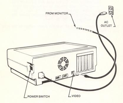
Connect the computer's main power cord to the main system unit, and plug the cord into a grounded 110 VAC 3-prong outlet. (Voltage requirements vary by country. Refer to the label on your computer.)
