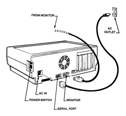
2b. Composite Monochrome Monitor Users: With the back of the unit facing you, connect the monitor's computer cable to the composite VIDEO connector on the back of your computer. Connect the monitor's power cord to an AC power source.
