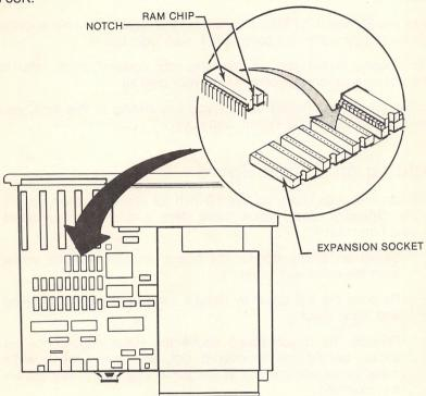
After you install the RAM chips, remove the jumper from staking pins E9 and E10. Refer to the System Unit Map diagram at the beginning of this chapter for the location of the 128K RAM Jumper. Install any other internal options you are adding at this time, and replace the shield and system unit cover.
