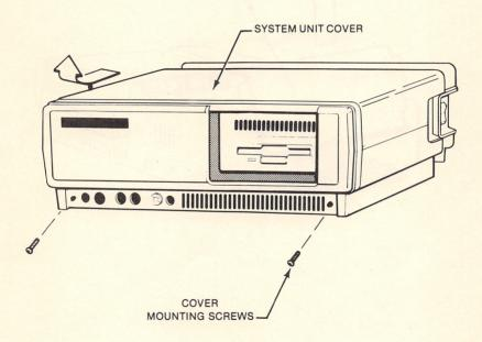
3. Remove the two screws holding the shield in place.
