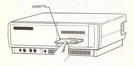
A drive's activity light is on whenever the diskette drive is reading from or writing to a diskette. Removing a diskette from a drive when the drive's activity light is on can destroy the data on the diskette.
