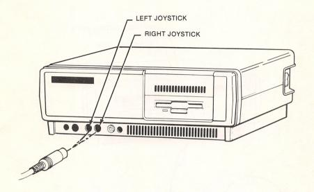
**Note:** The Right and Left indications on the joystick connectors are for reference only. Some application programs use these connectors interchangeably. If you use joystick software, and the program does not appear to function correctly, reverse the joysticks.
