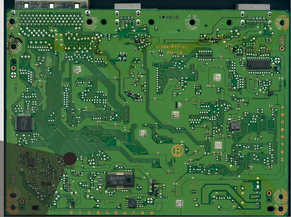
With the metal shield removed, flip the motherboard over to access the bottom.
