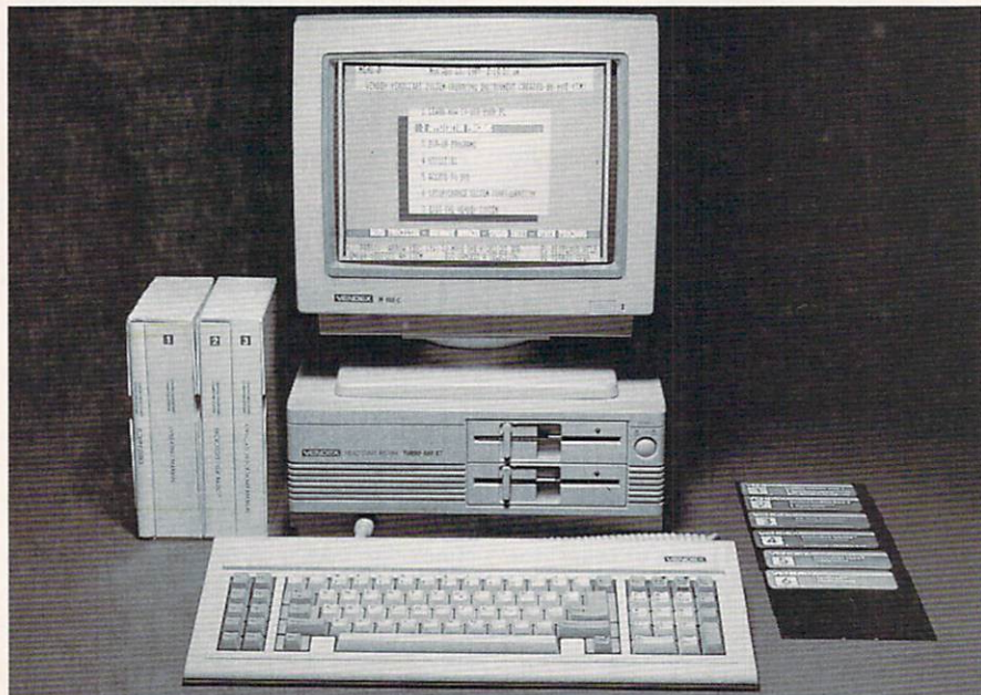
The Vendex HeadStart Turbo 888-XT comes with 512K of memory, a monochrome monitor, two 5.25-inch floppy disk drives, and five software packages.
